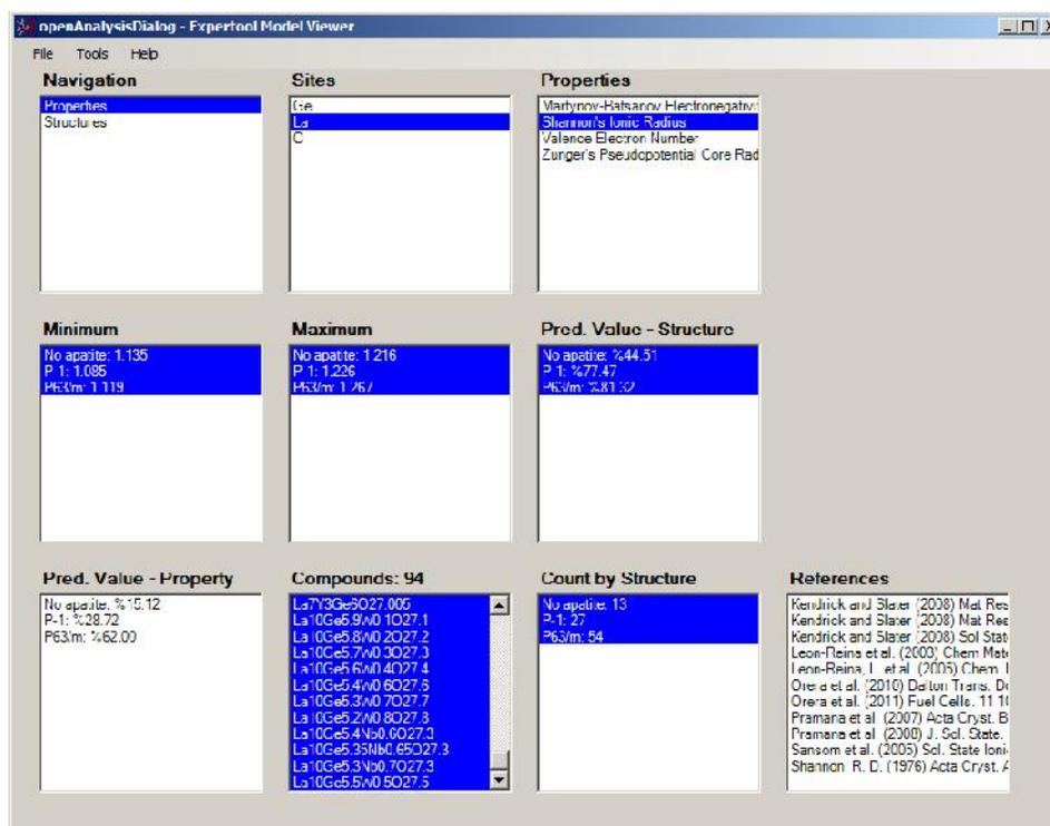
The “Pred. Value – Structure” window displays the range the property has for the given structure, as a percentage of the overall range of the property across the sample. The smaller the range, the more predictive the structure is of the property.
